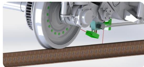
The construction can be adapted for use on most rail-based vehicles and can be adjusted for various track gauges. The system incorporates a suspension system to protect the Tribometer from railway vibrations and all sensing equipment mounted under the train bogie possess a IP54 rating or higher.
